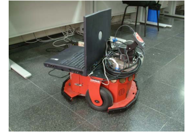
Fig. 7: Mobile robot and active camera.
