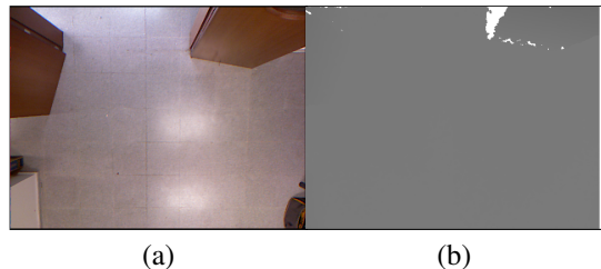
Figure 1. (a) RGB and (b) depth images. Observe in the depth image the artifacts depicted in white.
